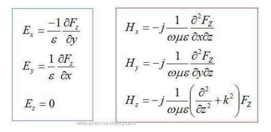
We can write the allowable field configurations for the TE (transverse electric) modes within a waveguide:
