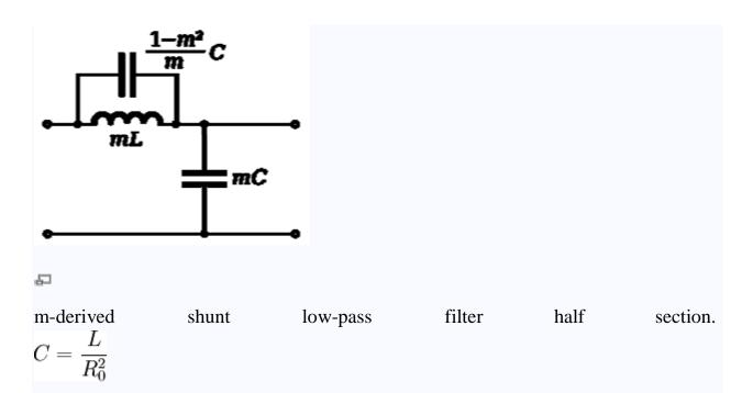
The building block of m-derived filters, as with all image impedance filters, is the "L" network, called a half-section and composed of a series impedance Z, and a shunt admittance Y. The m-derived filter is a derivative of the constant k filter. The starting point of the design is the values of Z and Y derived from the constant k prototype and are given by
