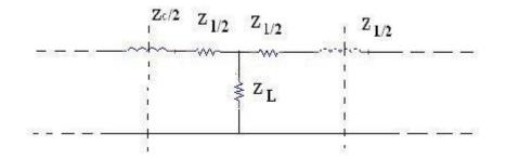
The section line may be replaced with an equivalent T section having symmetrical series arms. Adopting the notation of filter circuits one of these series arms is called  $Z_1/2$  and is
