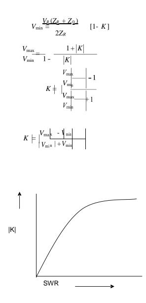
This figure shows the relation between standing wave ratio S and reflection coefficient
