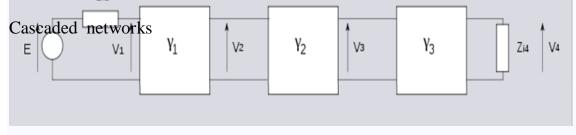
Three networks with arbitrary propagation constants and impedances connected in
