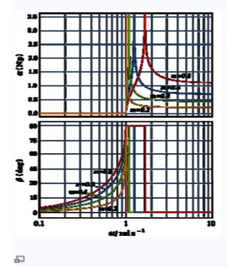
m-Derived low-pass filter transfer function for a single half-section
