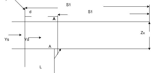
Since the input conductance of the of a line is S/R0 at a voltage maximum and S/R0 at a voltage minimum, then at some intermediate [point A the real part of the input admittance
