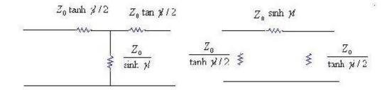
A  $\pi$  - section equivalent for the line may likewise be determined from the terminal measurements.
