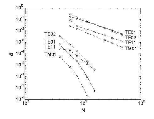
Figure 7: Convergence to the analytical result: relative frequency deviation Delta f versus the number of mesh intervals  $(N=N_s=N_theta)$  for the eigenmodes
