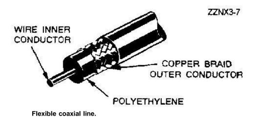
Because of the high-frequency losses associated with rubber insulators, polyethylene
