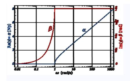
The transfer function of a constant k prototype low-pass filter for a single halfsection showing attenuation in nepers and phase change in radians.
