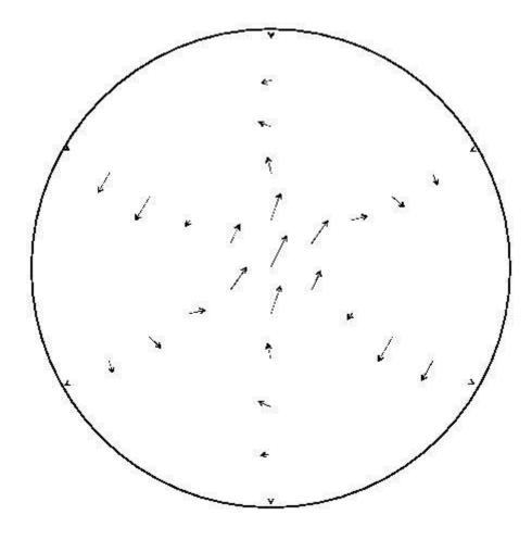
Figure 5: Re(A\_perp) for an eigenmode TE\_11 calculated with CFEM.
