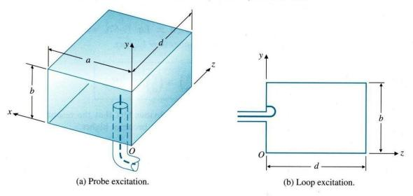
Resonant frequency of rectangular cavity resonator
