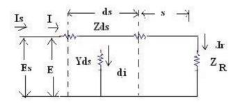
Hence the line current around the loop is not a constant, as is assumed in lumped constant circuits, but varies from point to point along the line. Differential circuit equations that describes that action will be written for the steady state, from which general circuit equation will be defined as follows.
