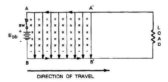
In figure 3-7, a battery is connected through a relatively long two-wire transmission line to a load at the far end of the line. At the instant the switch
