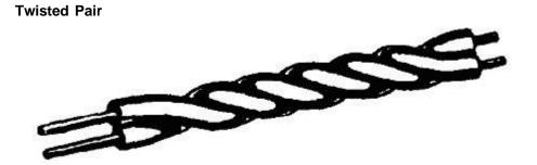
The TWISTED PAIR transmission line is illustrated in figure 3-11. As the name implies, the line consists of two insulated wires twisted together to form a flexible line without the use of spacers. It is not used for transmitting high frequency because of the high dielectric losses that occur in the rubber insulation. When the line is wet, the losses increase greatly.
